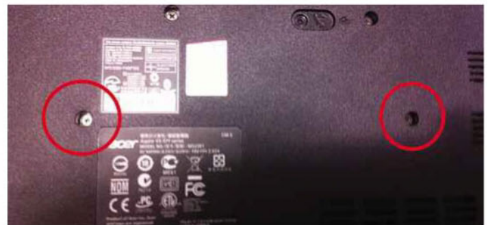
▲ Two screws need to be removed from the underside of the Acer V5-571 before the keyboard can be removed
